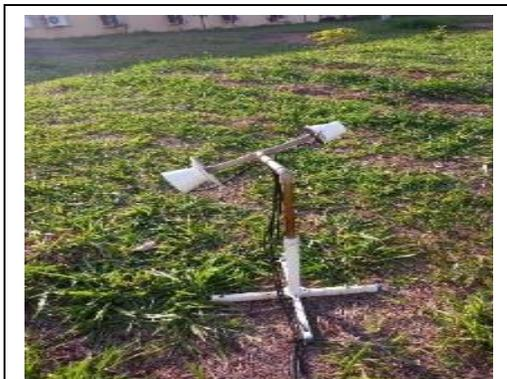
Figure 8. Radiometers for incident and reflected radiation.
