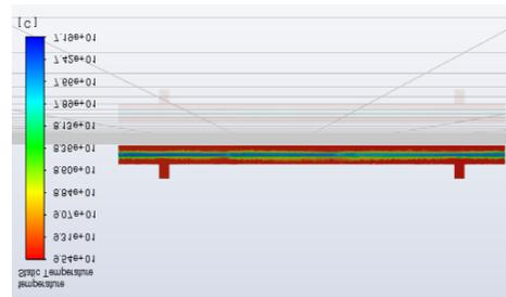
Figure 19. Temperature contour of irregular-Shaped tube heat exchanger.
