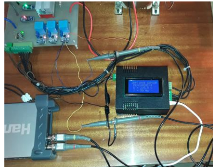
Figure 11. Measuring the output voltage and checking voltage on the sensor by using oscilloscope.
