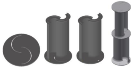
Figure 4. Assembly of the structure of the Savonius turbine with its 2 stages, straight blades and no shaft.
