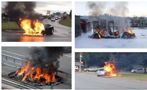
Figure 4. EV fires due to lithium dendrites.
