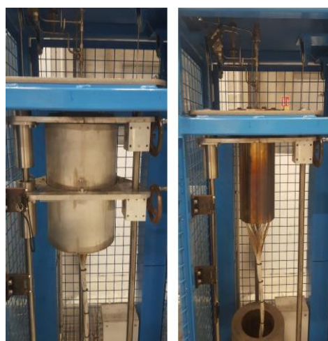
Figure 1. Batch reactor used for the hydrothermal liquefaction in the GEPEA Laboratory of DSEE department in IMT Atlantique.
