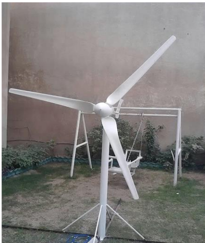
Figure 12. Wind turbine with NACA 4412 cross-section blades.
