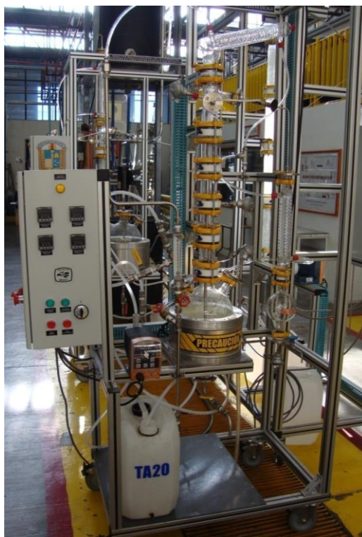
Figure 1. Experimental batch distillation column considered in this study.
