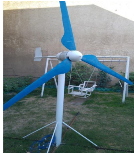
Figure 14. Wind turbine with EPPLER cross-section blades.
