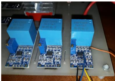
Figure 10. Implementation of voltage sensors in three-phase electronic system.
