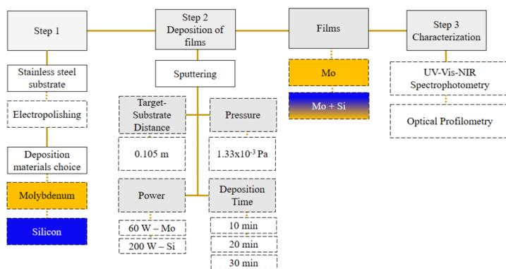
FIGURE 1. Experimental Process Flowchart.
