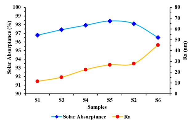
FIGURE 3. Correlation between the Ra parameter and the solar absorption of the films.
