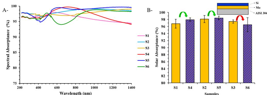
FIGURE 2. A- Absorbance spectrum of Mo and Mo/Si films deposited on electropolished substrates. B- Solar absorbances and their respective standard deviations.
