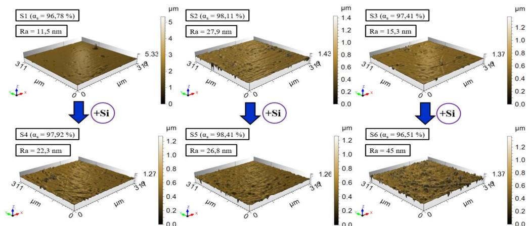
FIGURE 4. 3D Morphological profiles of films with single layer of Mo and with multilayer of Mo/Si.
