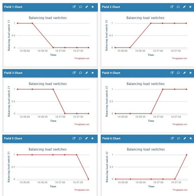
Figure 2: Real-time monitoring of IEEE 34-bus test grid topology – load balancing case study
