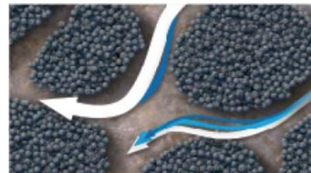
Figure 3. The HiWAY technique create stable, infinite-conductivity flow channels within fractures [9]
