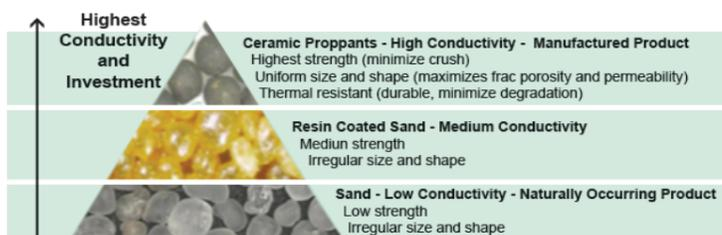
Figure 2. Scheme of proppant type [8]
