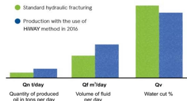
Figure 4. Diagram of production realized in the field "Itebej" in Vojvodina by different methods of fracturing [2]
