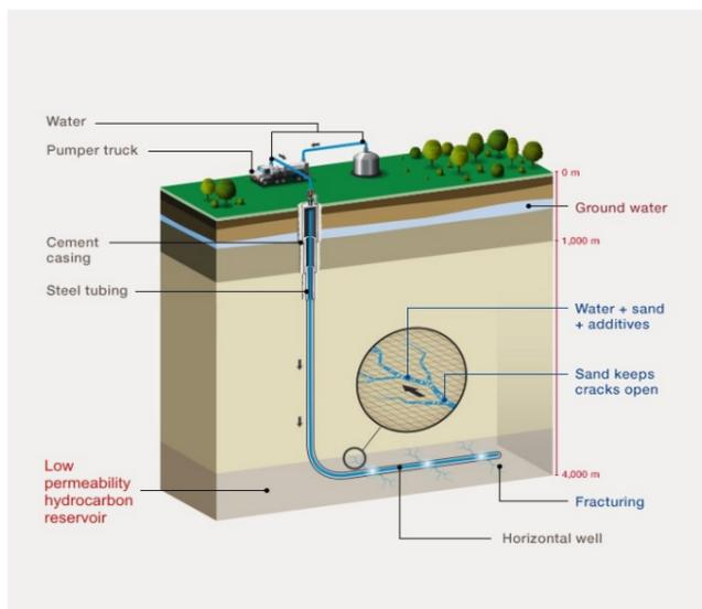
Figure 1. Hydraulic fracturing in a horizontal well [3]
