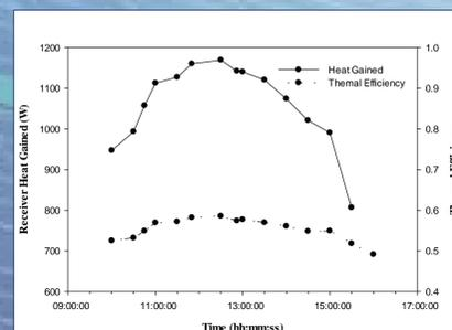
Fig.5. Variation of receiver heat gained ( $\dot{Q}_{net}$ ) and thermal efficiency of the cylindrical cavity receiver on 26th September 2016.
