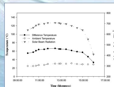
Fig.5. Variation of the solar irradiation, ambient temperature, and temperature difference between outlet and inlet of the cylindrical cavity receiver on 23th September 2016.
