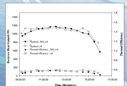
Fig.6 A thermal performance comparison between the silica/thermal oil nanofluid and pure thermal oil as the solar working fluid.
