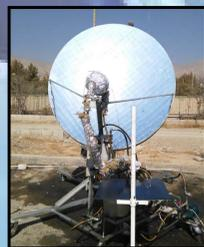
Fig. 1. The investigated parabolic dish concentrator with cavity receiver
