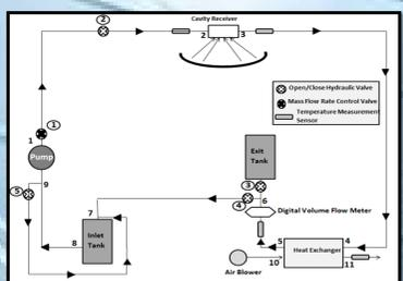
Fig. 3. Schematic of the hydraulic circuit
