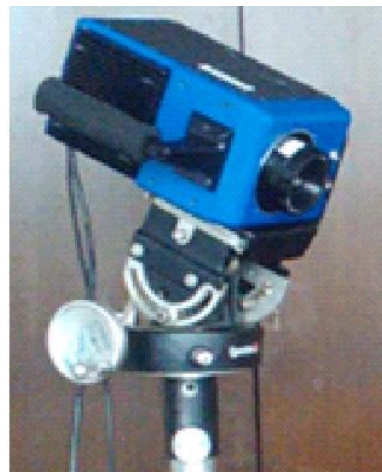
Figure 1. Non-commercial thermal camera FLIR SC720
