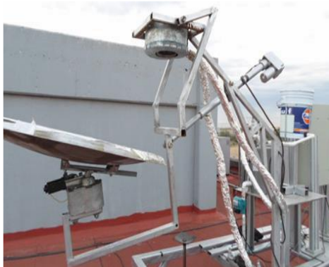
Figure 12. Solar tracker physically armed.
