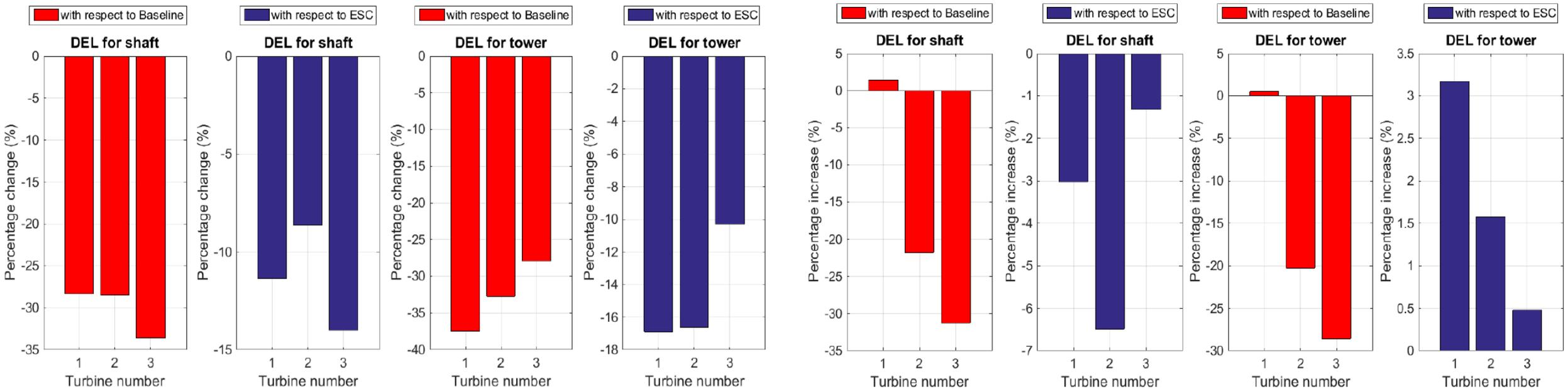
**Fig 6.** Percent change of mean value of moments for the shaft and the tower with respect to the baseline controller and ESC using additive penalty and multiplicative.
