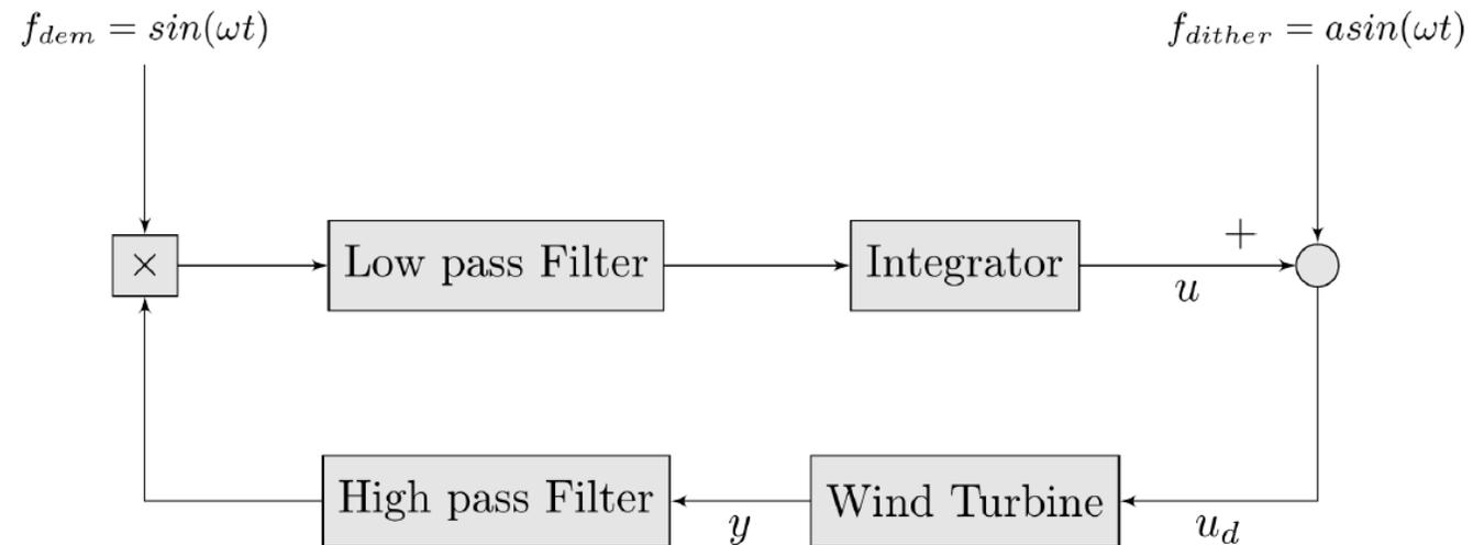
**Fig 2.** Block diagram of the ESC for a single wind turbine.
