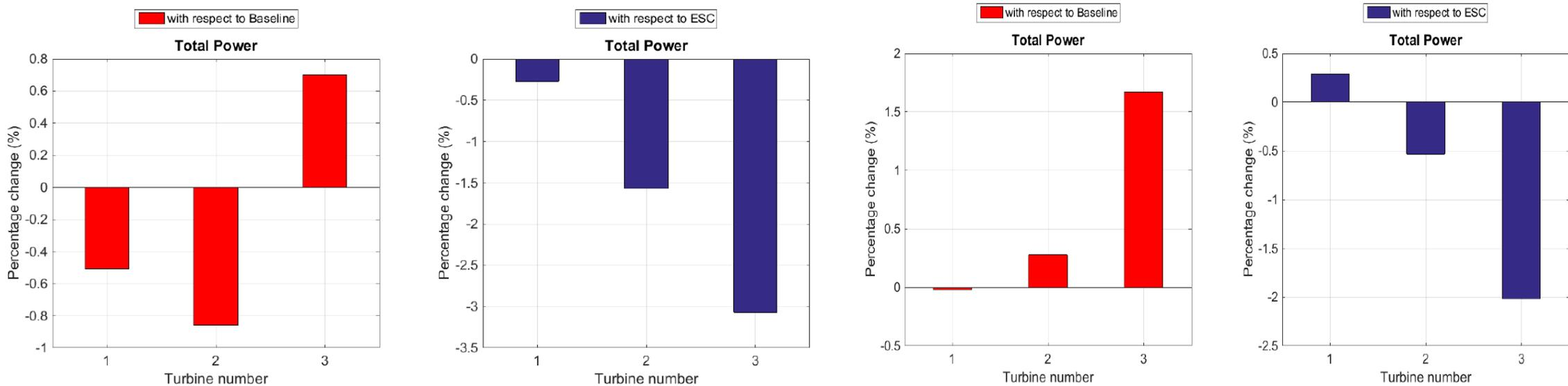
**Fig 7.** Percent change of total power with respect to the baseline controller and the ESC using additive penalty and multiplicative penalty based ESC load feedback.
