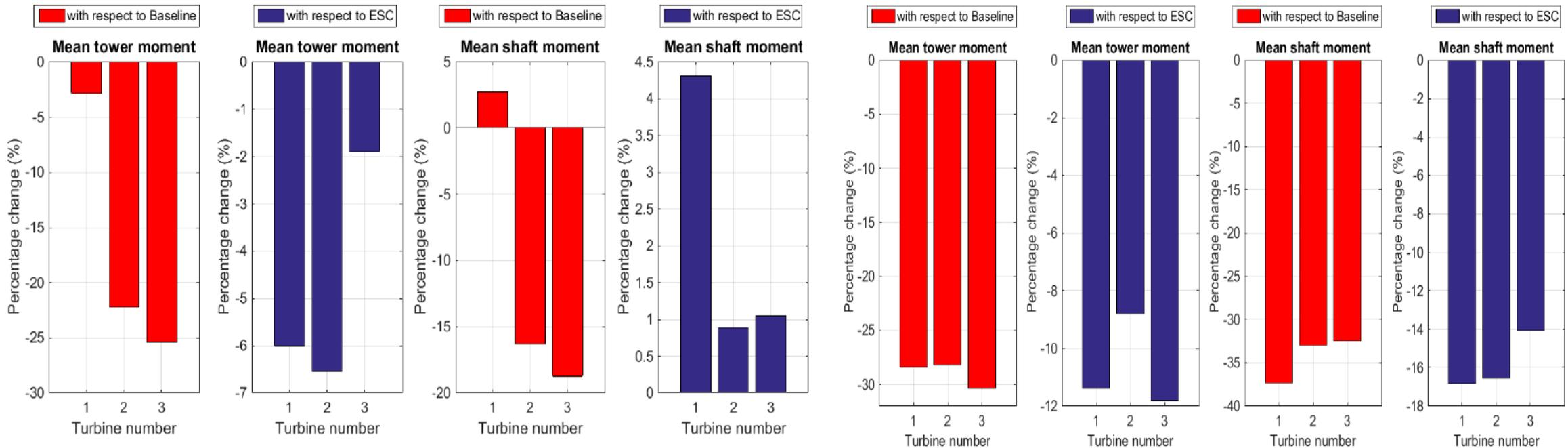
**Fig 5.** Percent change of damage equivalent loads for the shaft and the tower with respect to the baseline controller and the ESC using additive penalty based ESC and multiplicative ESC.
