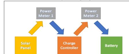
Figure 4(a). DC Charging Experimental Setup
