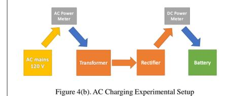
Figure 4(b). AC Charging Experimental Setup
