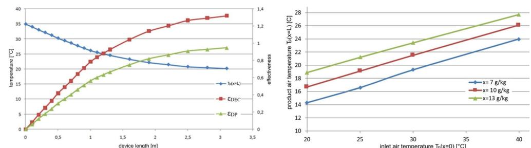
Figure 4: product air temperature, wet-bulb and dew point temperature effectiveness for various device lengths (left); product air temperature for different inlet air conditions (right)
