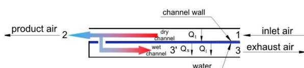
Figure 3: working diagram of counterflow indirect evaporative cooling
