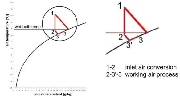
Figure 3: primary and secondary air conversion in the countercurrent cooling device
