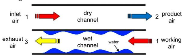
Figure 2: working diagram of indirect evaporative cooling
