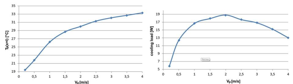
Figure 5: primary airflow velocity effect on the product airflow temperature (left); primary airflow velocity effect on the device cooling load (right)
