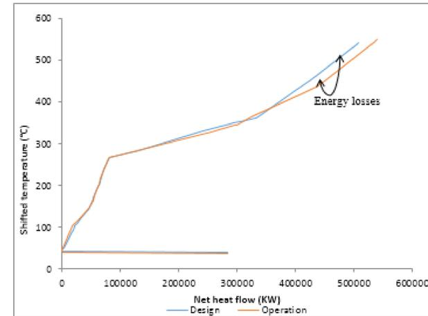
Fig. 2: Grand composite curves for the HEN under plant design and operation condition
