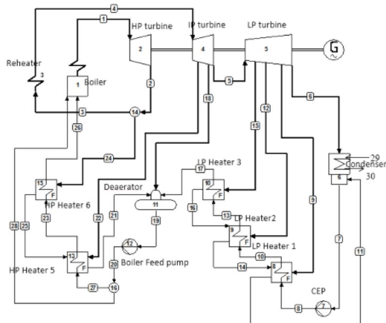
Fig. 1: Schematic of the Egbin TPP
