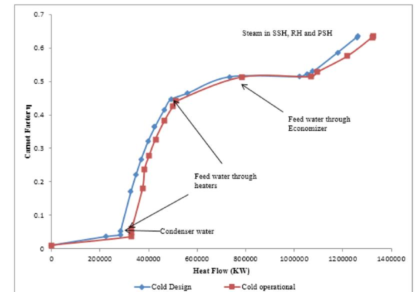
Fig. 5: Exergy grand composite curves for the HEN under plant design and operation conditions
