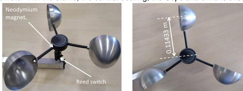
Figure 1. (a) Anemometer assembly; (b) Dimensions.
