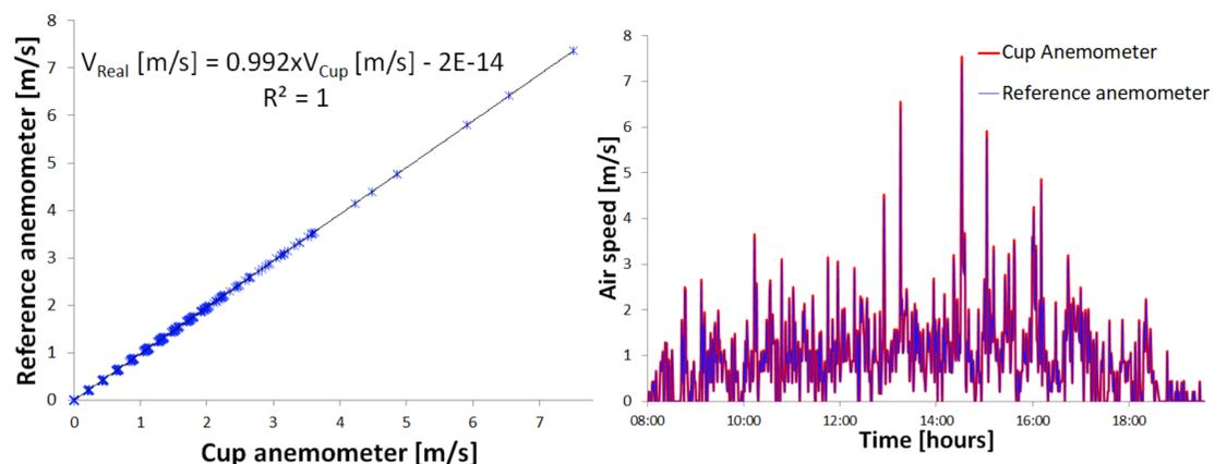
Figure 4. (a) Calibration curve; (b) Air speed comparison curve.
