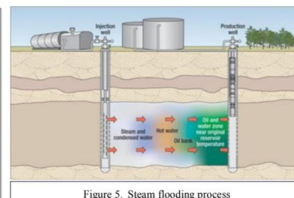
Figure 5. Steam flooding process
