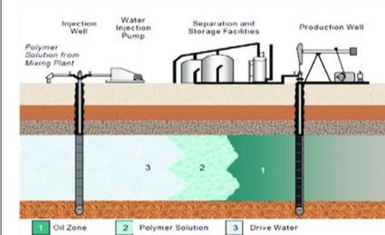
Figure 7. Polymer flooding
