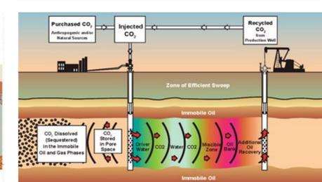
Figure 8. CO<sub>2</sub> injection "water alternate gas" method
