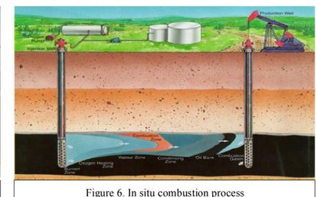
Figure 6. In situ combustion process
